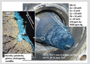
FFCV= Fluid Flow Control Valve covered with 800 gr of metals which precipitated in one year, concentration of the precipitated metals: Zn 20 wt%, Fe 9 wt%, Cu 23 wt%, Pb 15 wt%, S 22 wt%, 570 ppm Au, and 9200 ppm Ag. © **Vigdís Harðardóttir Ph.D Thesis University of Ottawa 2011**.
